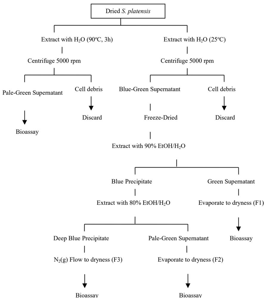
**Figure 1.** Flow chart of the extraction process of *S. platensis* to obtain the aqueous extract
