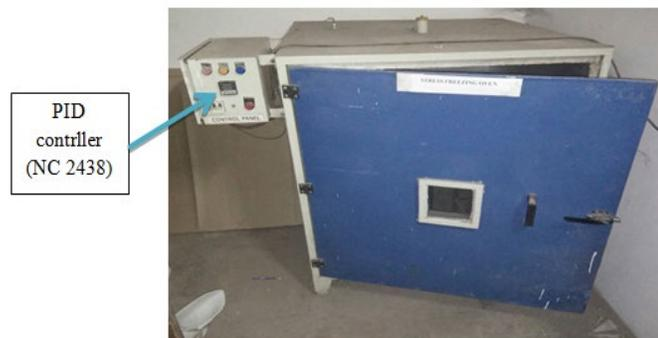
Figure 4. Stress freezing oven
